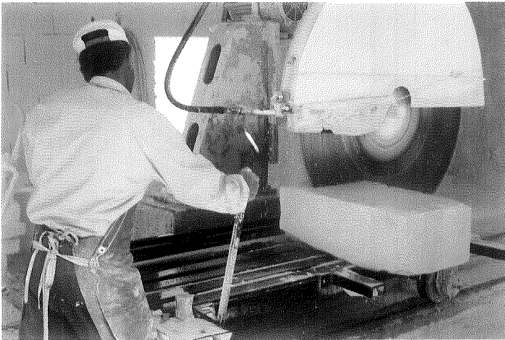
333) Rock cutting in stonework shop. (Photograph by: S. Sabri Kürkçüoğlu).
